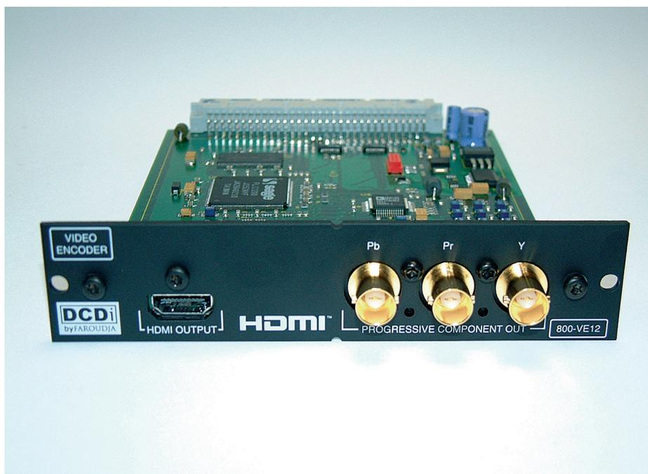
HDMI and Progressive outputs for Meridian's 800 optical disc player
