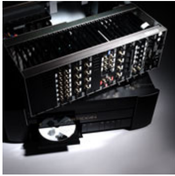
The 861 processor can be fully equipped with a variety of input/output sockets
