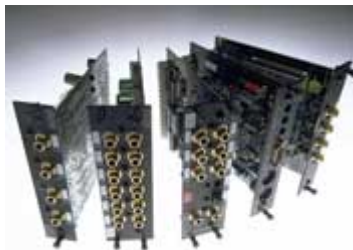
Both the 800 and 861 are configured like a computer with removable cards
