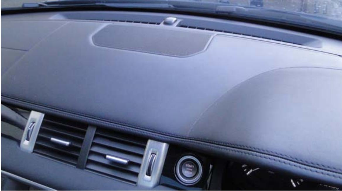
A key component here is the centre channel speaker, something that originally sprang out of Meridian's home-theatre technology. "With normal two-channel stereo audio you're effectively hearing a phantom centre channel. If you put a real speaker there, it does two things. First, it provides a fundamental point source. The other thing is that you get a consistent sound source regardless of where you are sitting."
