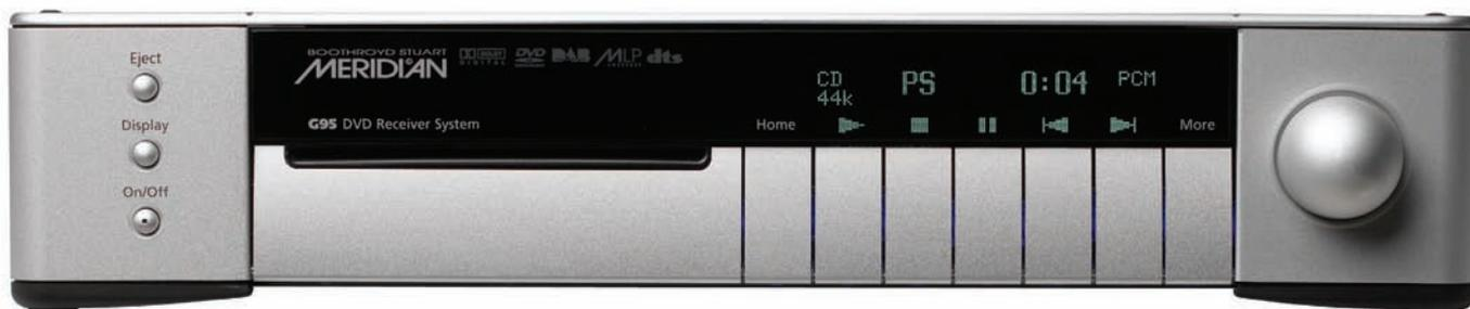
G95 front panel showing slot-loading drive
