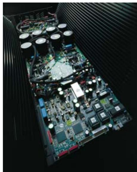
driver is individually equalized to provide a greater linearity than would normally be possible by traditional passive means. All of this is done with custom written software developed over many years by Meridian's staff of DSP engineers.
