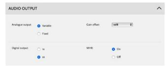
**Analogue output**: Choose **Variable** if the 218 is to control the volume of the analogue outputs, or **Fixed** if the analogue outputs are connected to a preamplifier with its own volume control.
