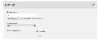
**Startup volume**: Specifies the initial volume for the analogue outputs (if variable) and, if the 218 is a Controller, sent on Meridian Comms for other products. The start volume is set when the 218 is first powered up, and a few seconds after going into standby.
