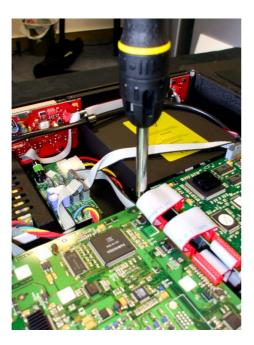
3. Disconnect the four looms which connect the PCB electrically to the other parts of the unit. There are three grey and red "Micromatch" looms and one grey power loom.
