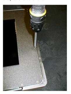
Poistion the unit so that the rear-panel is accessible. Remove the eight T10 Torx screws and
