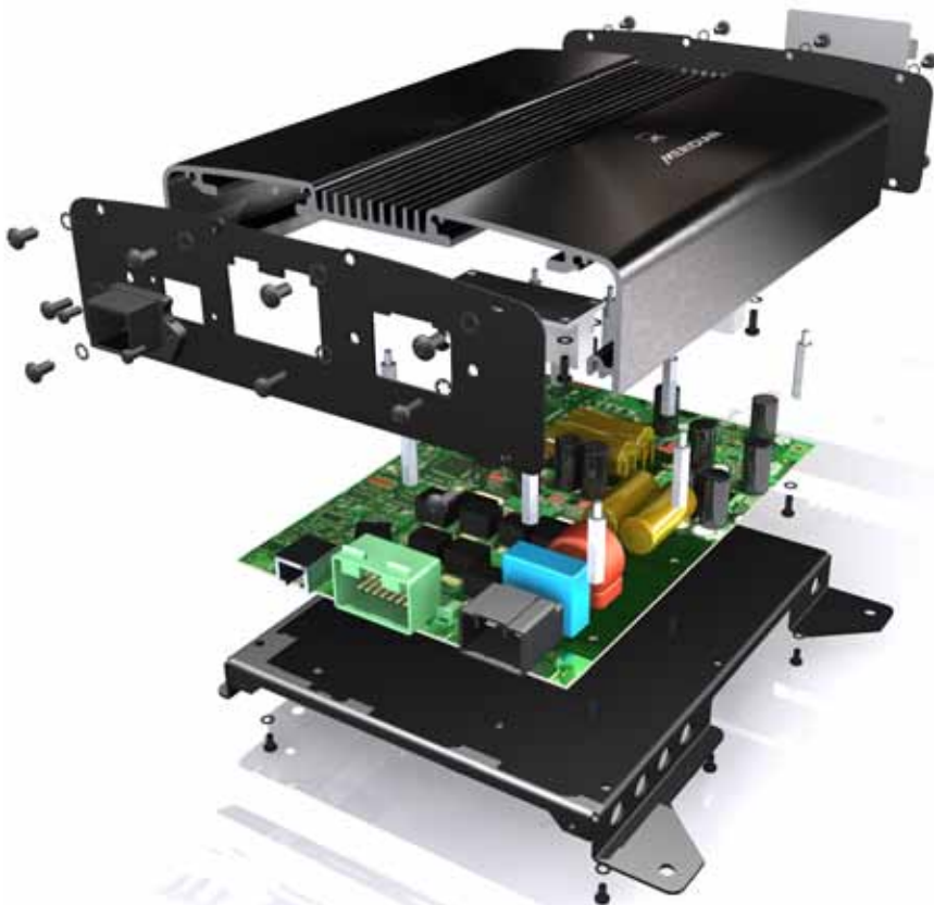
Exploded view of the amplifier/DSP unit
