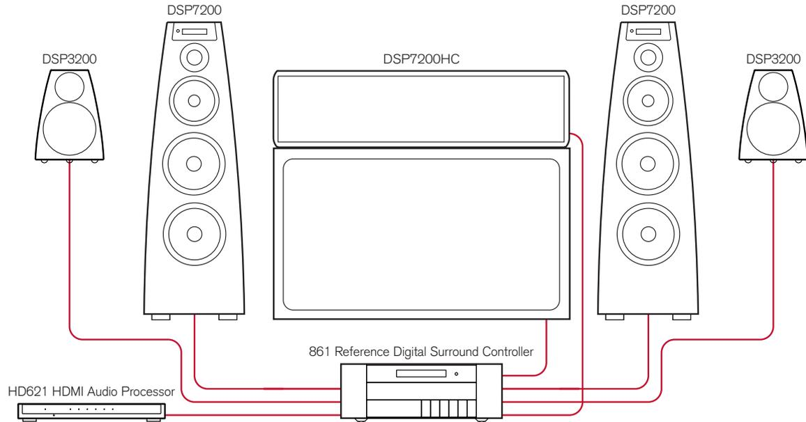
Up to seven Meridian DSP loudspeakers can be used in conjunction with a Meridian surround controller, such as the 861 Reference Digital Surround Controller, to create a digital surround system with superb music and cinema sound.
