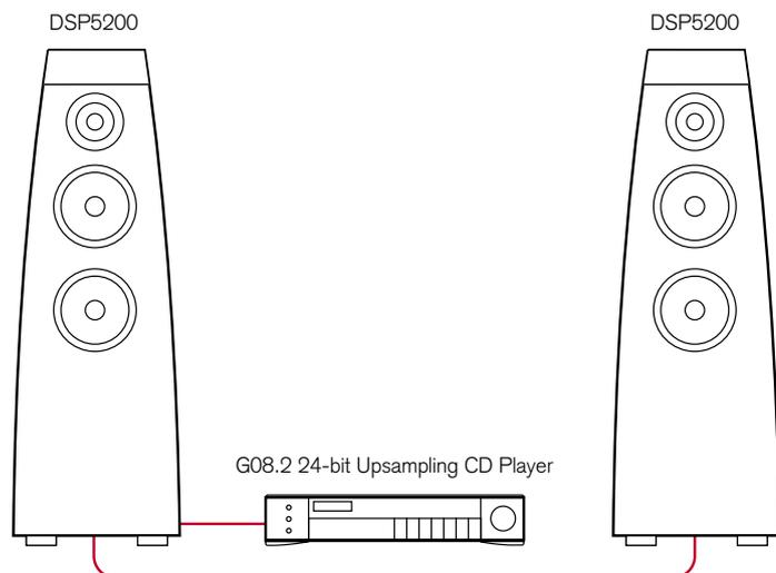
Meridian DSP loudspeakers include DSP volume and tone controls, and can be connected directly to up to two digital sources, such as the G08.2 24-bit Upsampling CD Player, to create an extremely compact high-quality music system.
