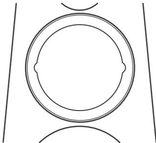
Hold the ring by one of the indentations by depressing the grille fabric with your thumb, and then wiggle the
