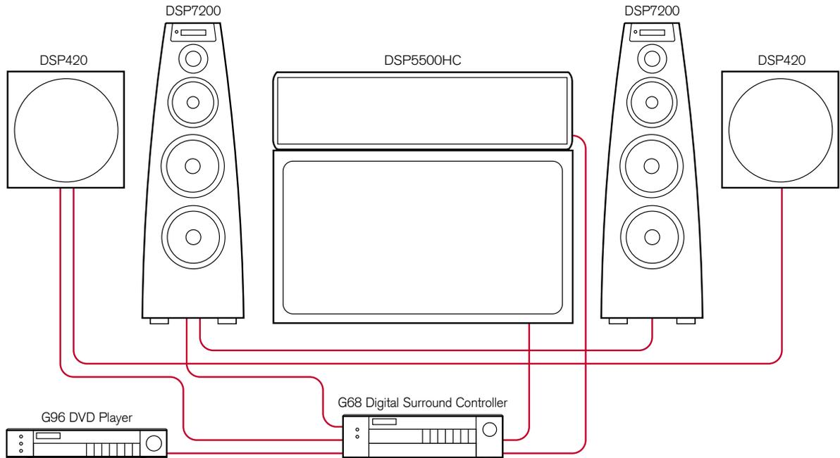
Up to seven Meridian DSP loudspeakers can be used in conjunction with a Meridian Surround Processor, such as the G68 Digital Surround Controller, to create a digital surround system with superb music and cinema sound.
