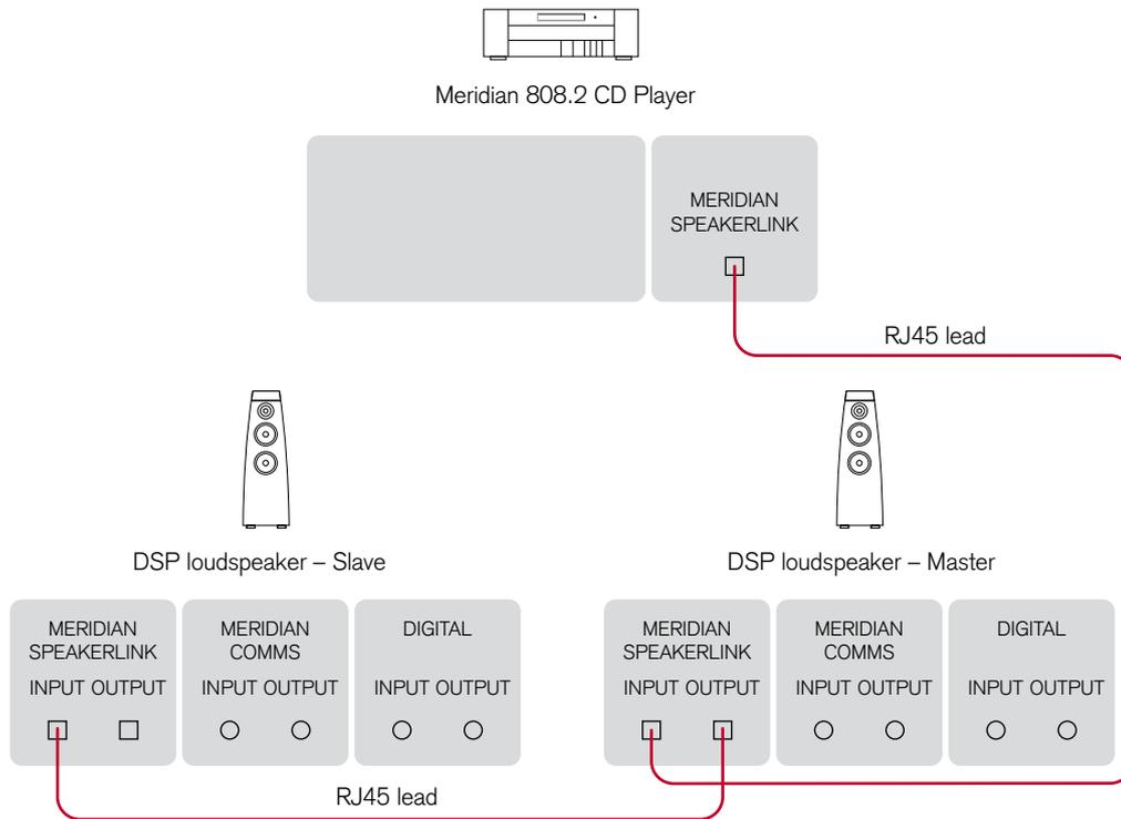
You can create a complete system by connecting a pair of DSP loudspeakers directly to a digital source. The DSP loudspeakers include volume, balance, and tone controls allowing you to control the system using the MSR+.
