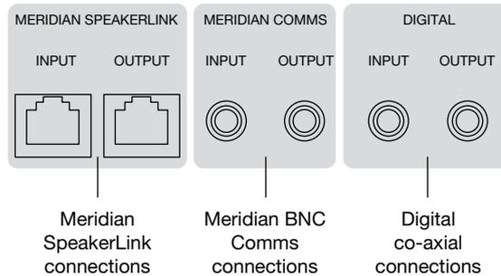
You can connect to the DSP loudspeakers using either the RJ45 SpeakerLink connectors, or the Meridian BNC Comms and digital co-axial connectors.
