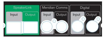
The DSP8000 now includes SpeakerLink – a new interconnection system that links Meridian components with a single CAT 5 cable, for the ultimate in easy installation.
