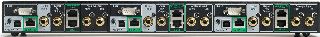
Distributor 3 includes three identical, independent zones sourced by analogue, digital or SpeakerLink inputs
