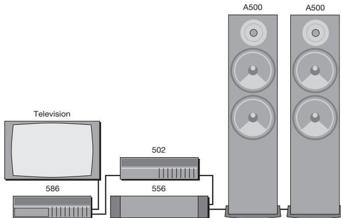
The 586 DVD Player provides a two-channel analogue audio output, normally encoded in Dolby Surround, to allow direct connection to an analogue pre-amplifier such as the 502 Analogue Controller.
