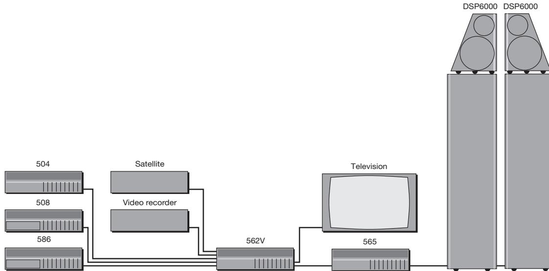
The Meridian 562V Multimedia Controller is the ideal control unit for use as the heart of a versatile multimedia system, giving flexible control of video, digital audio, and analogue audio sources. It provides direct digital inputs for digital sources, such as the 508 Compact Disc Transport and DVD sound from the 586 DVD Player.
