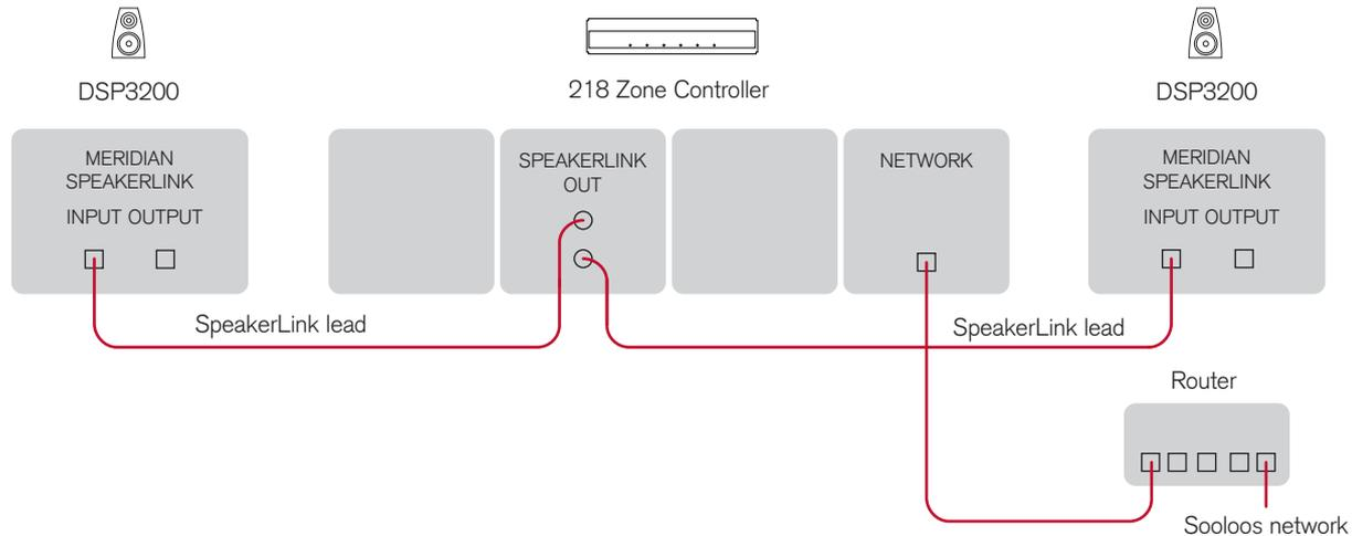
This is a simple, standalone system replaying audio from a Sooloos system, using the Sooloos UI to control the volume.
