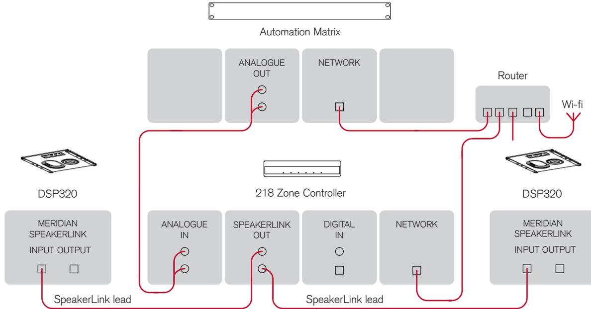
This layout is intended to play back audio in a single zone as part of a larger, whole-house, automation system. The 218 is located in a central rack along with the automation system's audio matrix.
