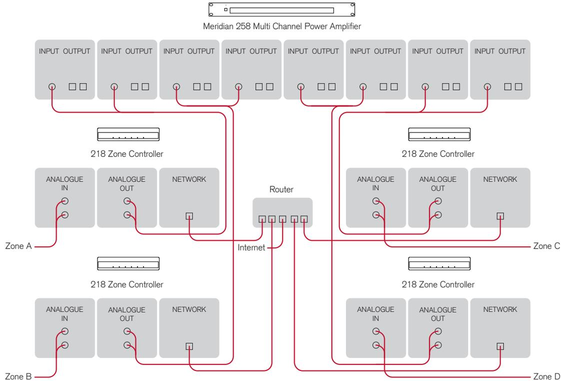
In this system multiple zones are each controlled by a separate 218, using a 258 Multi Channel Power Amplifier to drive the loudspeakers in each zone. The 218s and 258 power amplifier are located in the central rack along with any automation equipment.
